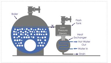
This drawing shows Flash Steam recovered for the steam distribution system and the hot blow-down condensate flowing into a heat exchanger to pre-heat incoming makeup water.
