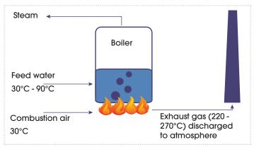
The graphic presents a process flow diagram of a typical industrial boiler system. Combustion for heat generation begins in the boiler burner system and the heat is transferred to the water in the boiler. The boiler produces steam and hot water for industrial process applications. Boilers can utilize an economizer to preheat the process water before it is fed to the boiler using waste heat from the exhaust gas.
