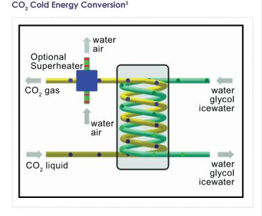
and warm glycol or water returning from the process to the refrigeration chillers can be used to vaporize the  $CO_2$  and the heat extracted from the warm stream will help lower energy usage as well. This heat recovery process will help lower energy usage and cost associated with the steam, hot water or electricity used to vaporize  $CO_2$ .
