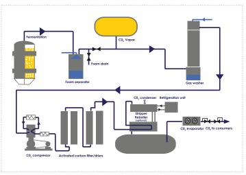
Traditional  $\rm CO_2$  Collection Methods and the Installation of  $\rm CO_2$   $\rm Stripper/Reboiler^2$
